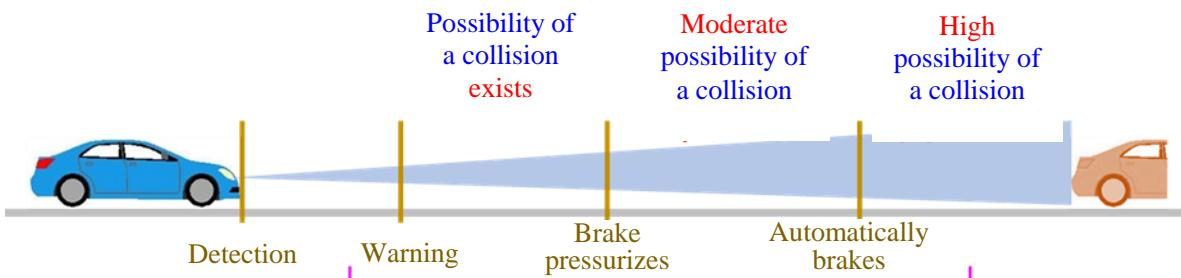
Fig. 1. Mechanism by which collision damage mitigation brakes operate
