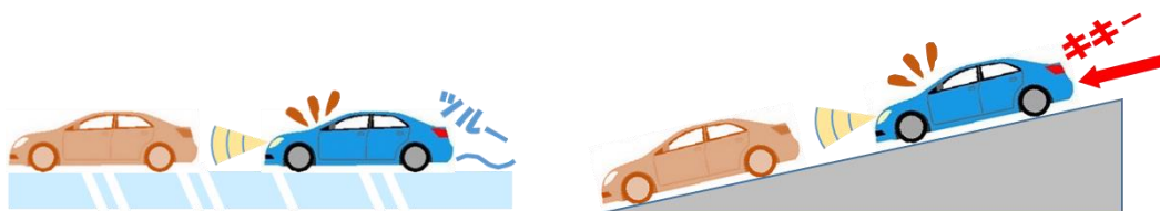
Fig. 14. Scenarios where the AEB tends to not be effective (Left: Slippery road surface; Right: Steep downhill)
