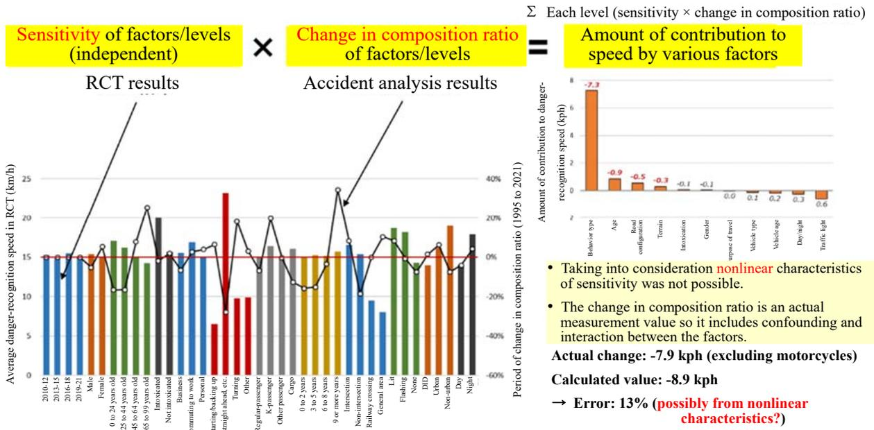
Figure B. Process of calculating amount of contribution of various factors to danger-recognition speed
