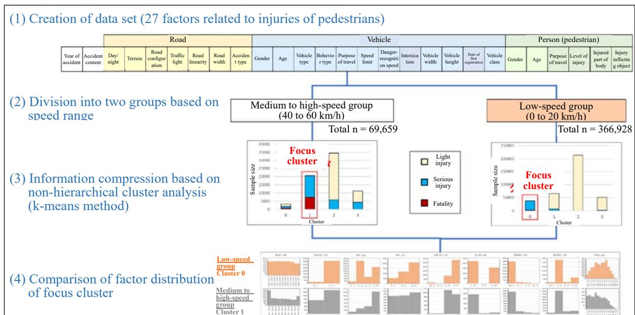
Figure 10. Procedure for analysis of factors that lead to fatalities & serious injuries in low-speed range
